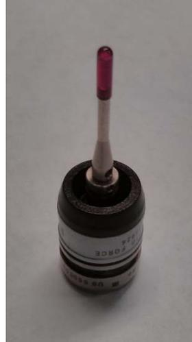
Figure 52 - CMM probe module and stylus
