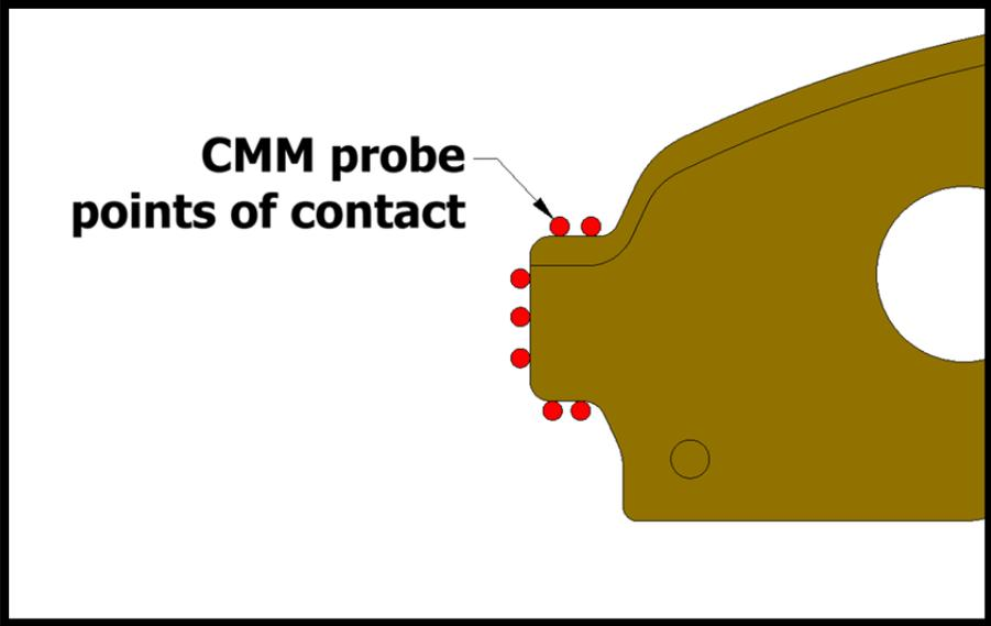
Figure 2 - CMM points of contact on the abutments (left abutment shown)
