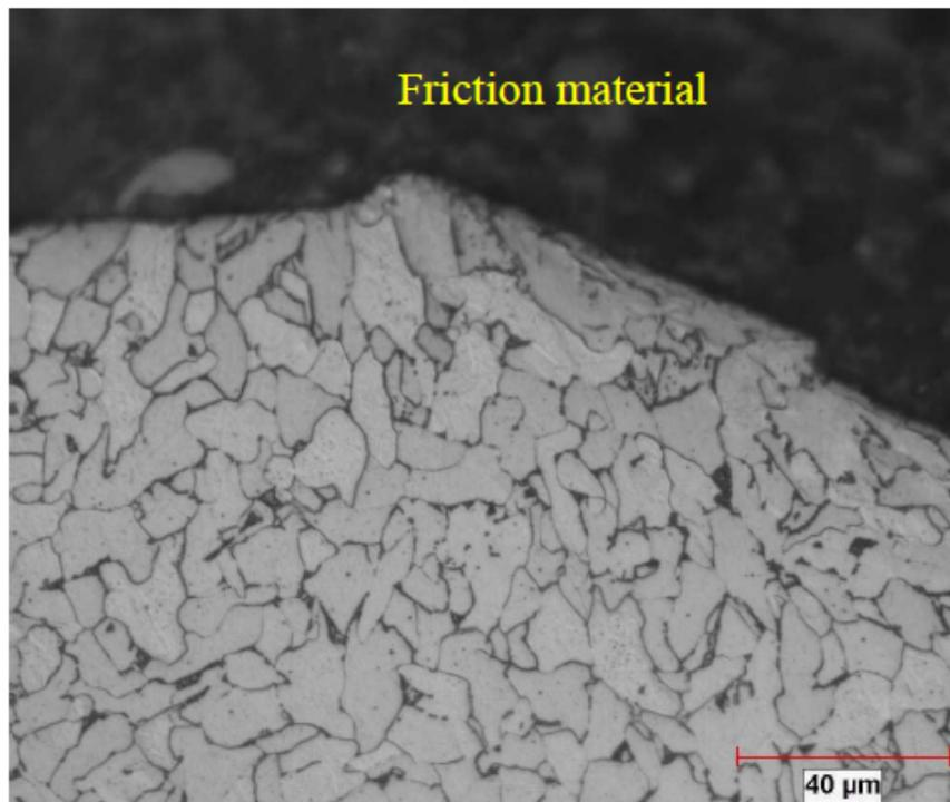
Figure 47 - Sample 7: Disc brake shoe - SAE 1010 HRPO, painted - Metallographic Microscope Image [6]
