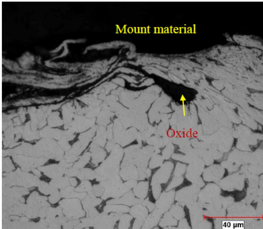
Figure 43 - Sample 2: Black steel, shot blasted - Metallographic Microscope Image [6]
