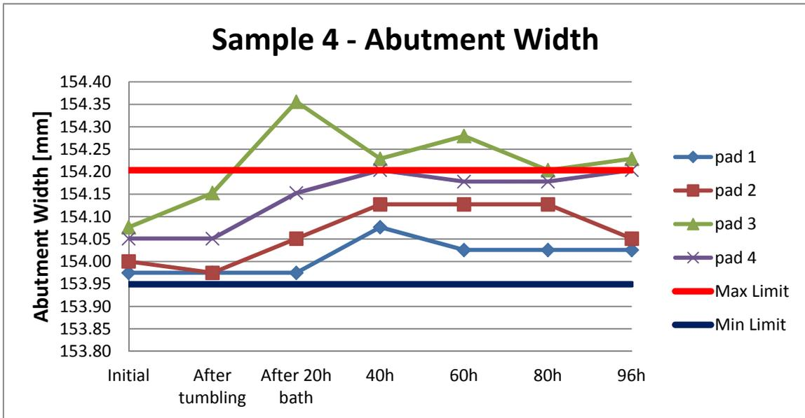
Figure 31 - Sample set 4 - Premium grade using zinc coated disc brake shoe
