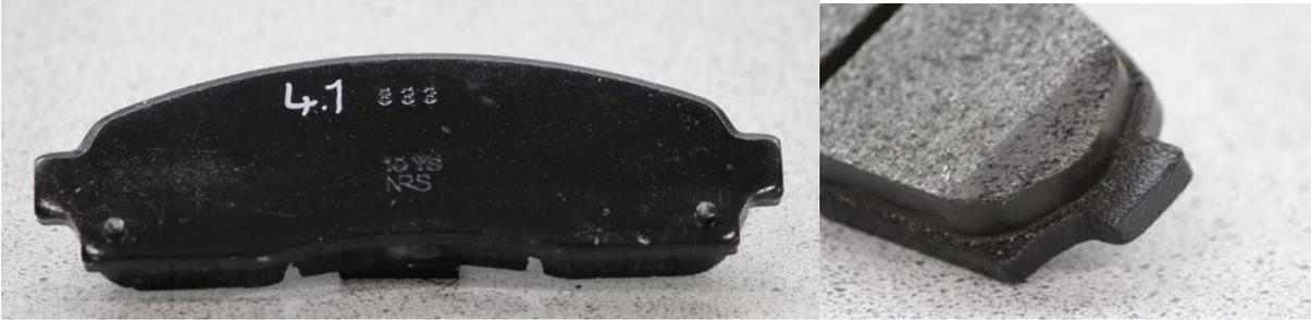
**Figure 5 - Sample 4.1 - Premium grade using zinc coated disc brake shoe (Initial)**
