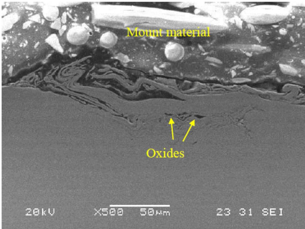
Figure 42 - Sample 2: Black steel, shot blasted - SEM Image [6]
