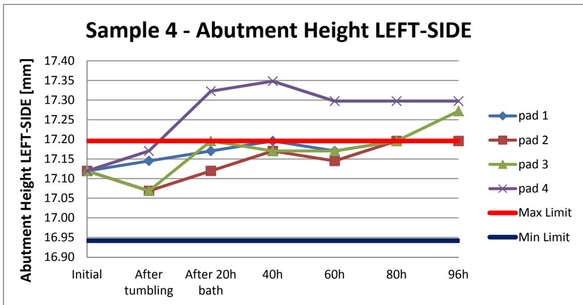
Figure 35 - Sample set 4 - Premium grade using zinc coated disc brake shoe
