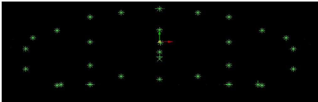
Figure 53 - Position of points taken with CMM probe for flatness
