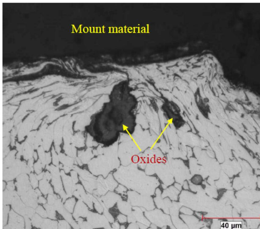
Figure 45 - Sample 3: Black steel, shot blasted with adhesive - Metallographic Microscope Image [6]
