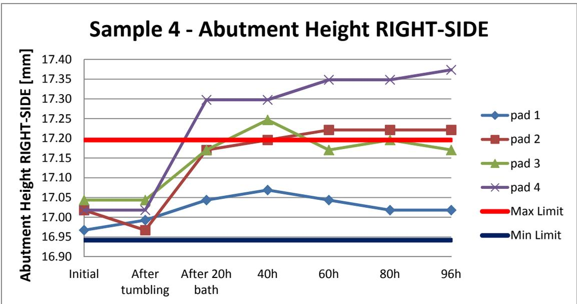
Figure 399 - Sample set 4 - Premium grade using zinc coated disc brake shoe
