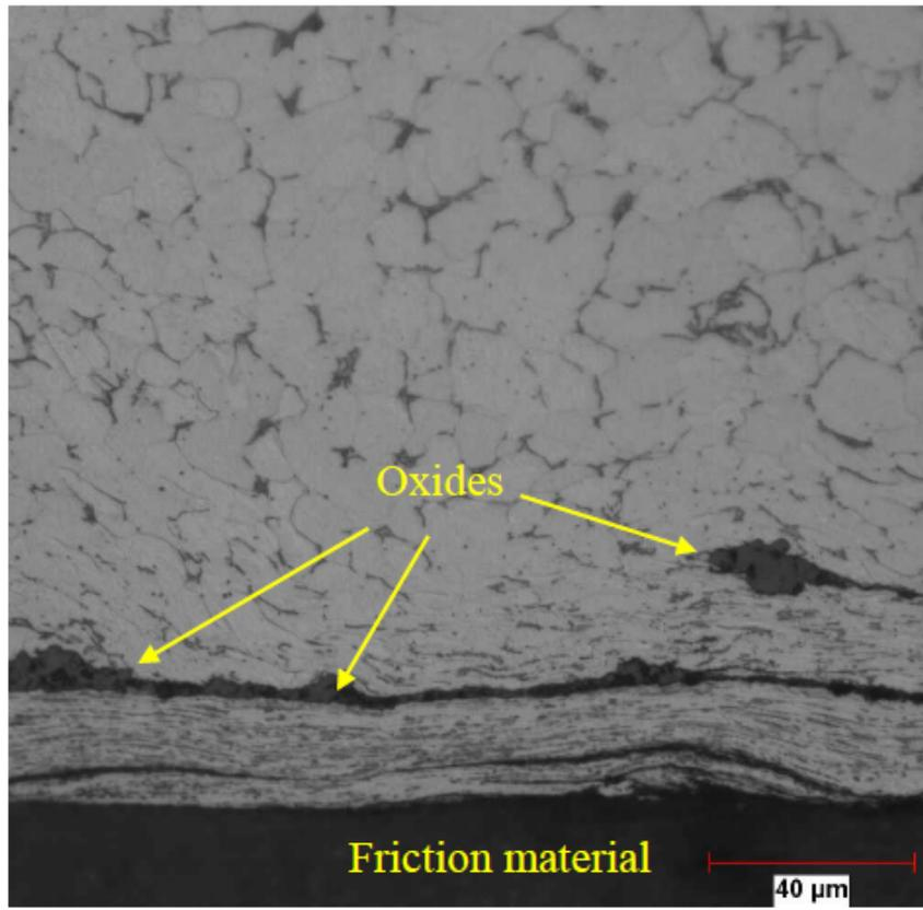
Figure 49 - Sample 8: Disc brake shoe - suspected black steel, painted - Metallographic Microscope Image [6]
